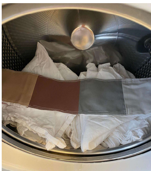
Figure 8. Loading procedure, showing folded filling material (cotton towels) with a stain strip on top.
